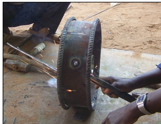
Picture 9: The wheel being welded showing the tire valve hole
