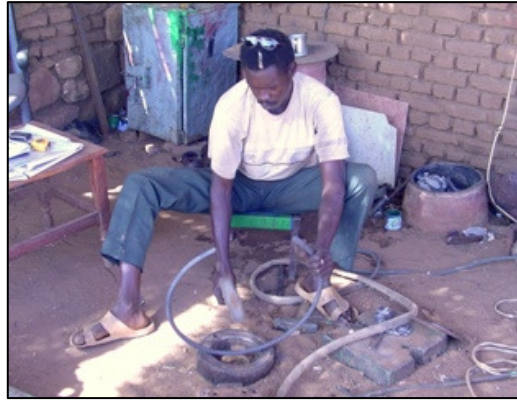
Picture 6: A Fabricator bends the metal bar (Part A) using a hammer and a bend former (i)
