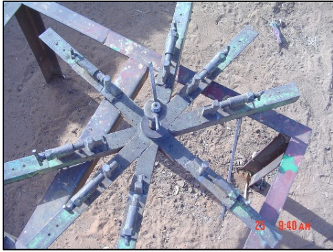
Picture 4: A completed wheel jig
