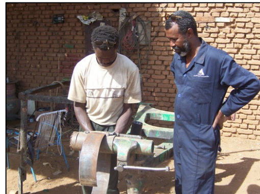
Picture 7: The fabricator bends the flat plate (Part B) using the bending tool
