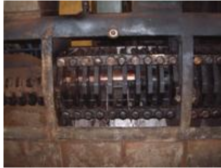
Figure 7: Typical view of cage or barrel of an expeller. Photo: Tony Swetman.
