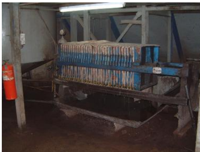
Figure 8: Typical filter press. Photo: Tony Swetman.
