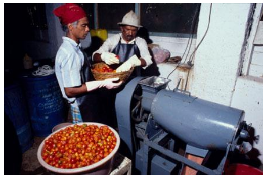
Figure 3: Tomato processing unit at Walewela, Sri Lanka. Putting tomatoes in the pulper. Photo: Practical Action / Zul.
