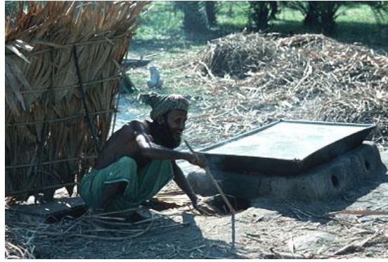
Figure 3: A simple open pan used for processing the juice extracted from the sugar. Photo: Neil Cooper / Practical Action.
