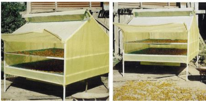
Figure 4: A typical solar drier developed in Bolivia
