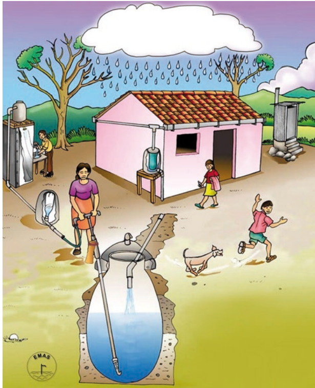
Figure 6.3 EMAS promotional material showing basic household water and sanitation technologies: rainwater harvesting with underground water storage tank; a manual pump to lift water to a small elevated tank for a shower and washing sink; and a ventilated latrine Source: J. Buchner, EMAS, 2010
