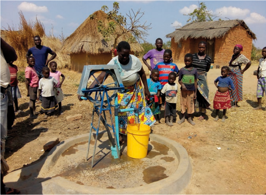
Photo CS.6.2 Family borehole and rope pump installed by Jacana, in Eastern Province, Zambia Source: Photo: Rik Haanen, Jacana
