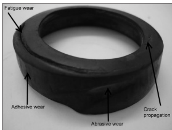
Figure 9.2 Wear mechanisms of a worn piston seal
