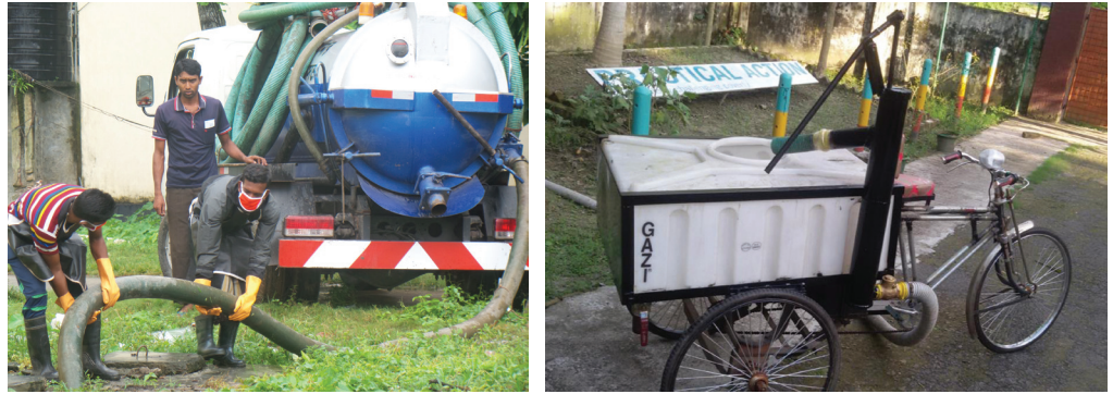
Desludging technologies used by Khutibari Cleaners Cooperative, Faridpur Source: © Practical Action Bangladesh
