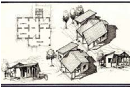
Figure 11.1 Drawing of house plan showing the design principle of having the same floor plan but different roof shapes
