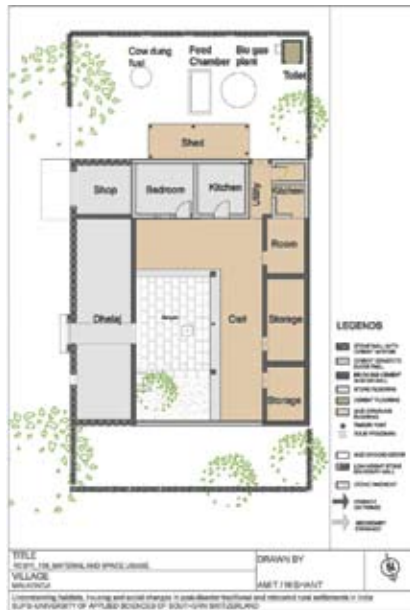
Figure 3.4 Example of extensions carried out to a core house in Malkondji
