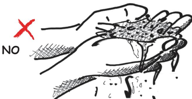
Concrete must be used in less than 90 minutes.
