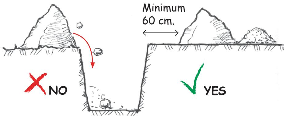
**WARNING:** dig until you reach firm soil and then build the foundation to the proper width.
