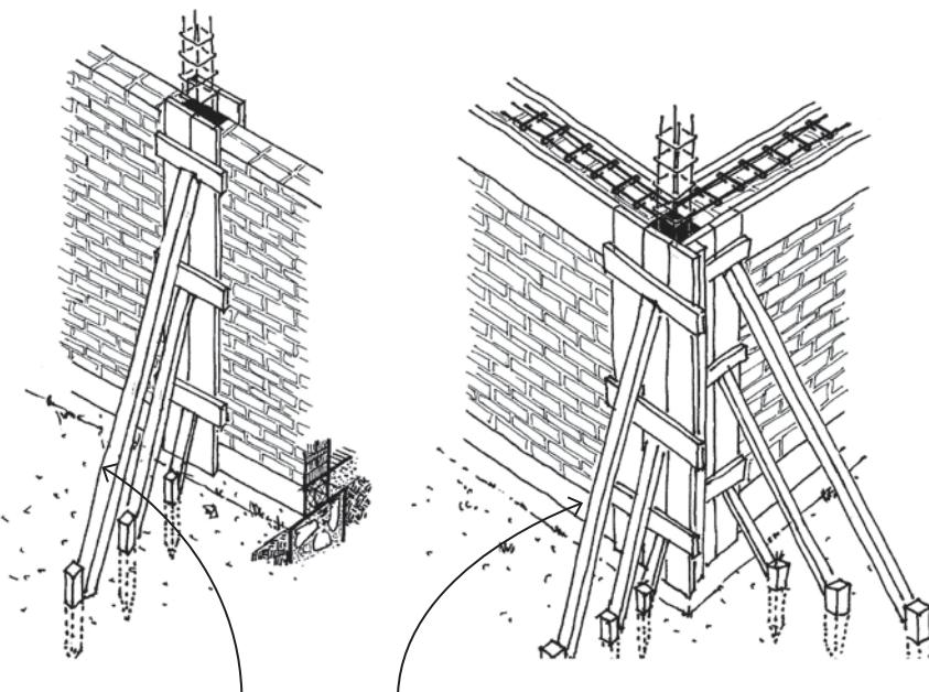
Formwork must be well braced.
