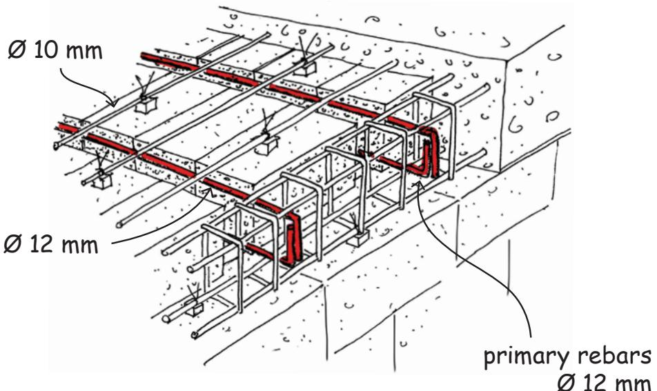
To ensure a good connection, it is important to insert the hooked slab rebars deep into the bond beam.
