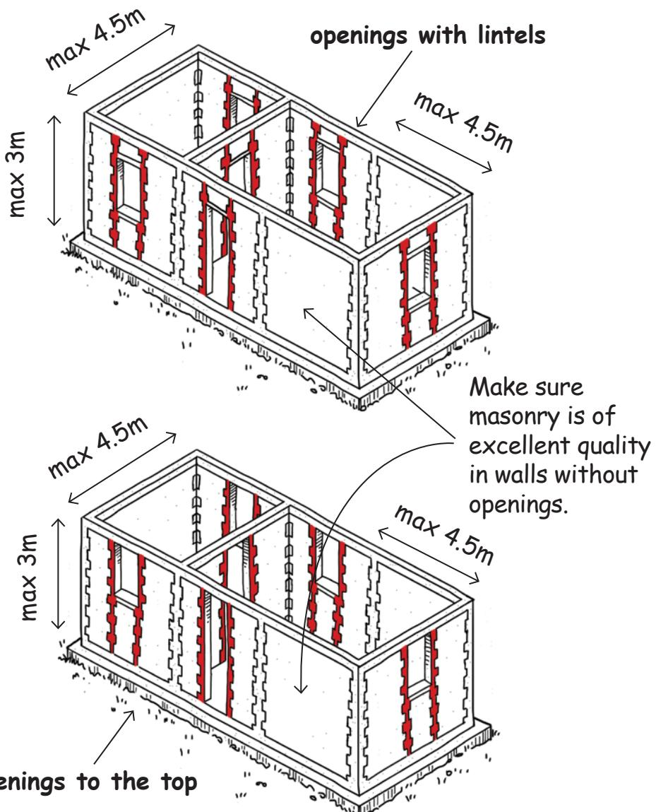
Place a vertical reinforcement on each side of every opening.
