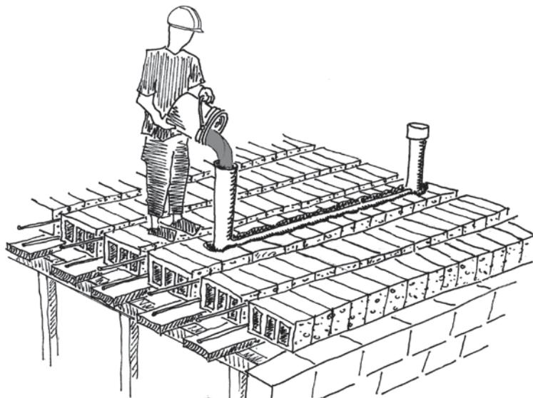
Test watertightness of the pipes by filling them with water and wait for four hours.
