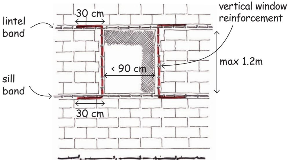
Hook the window reinforcement and lap 30 cm with the seismic band reinforcement, into the stirrups.
