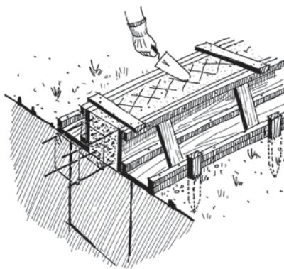
Roughen up the top surface of the plinth beam to increase bonding of the mortar for the wall.
