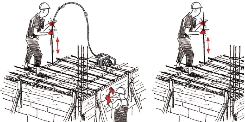
Compact the concrete with a vibrating needle or, if not available, with a steel rod and hammer.
