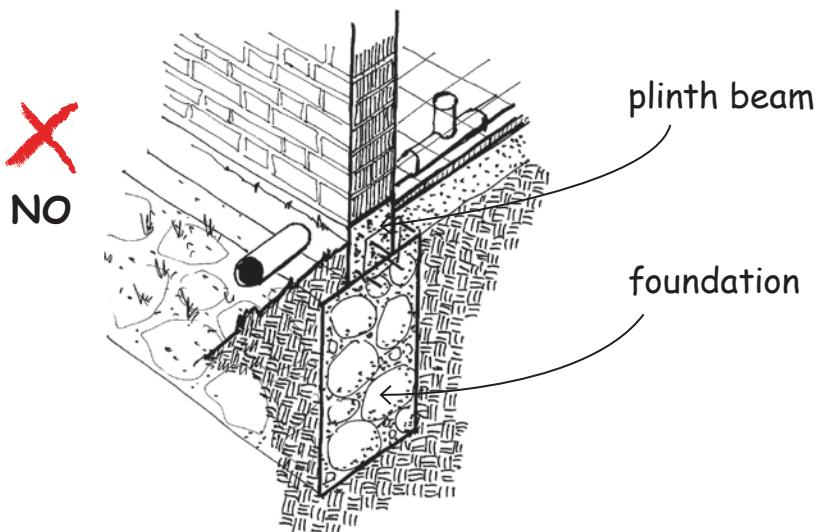
The pipe must not go through the plinth beam.
