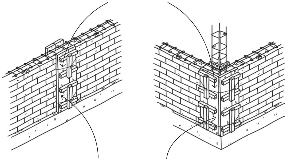
Attention: with this type of formwork wait until the masonry is solid or the wires will move the bricks.
