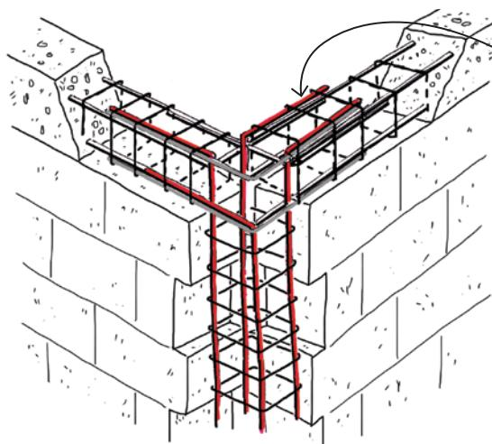
At the top of the wall bend the vertical rebars into the tie-beam.
