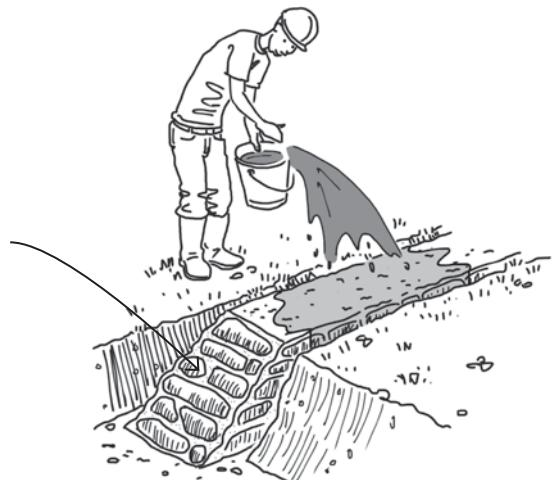
**Build a 'drainage pad' under the floor to block ascending humidity.**
