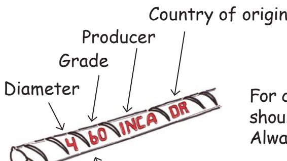
For confined masonry **Grade 60** should be used.
