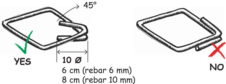
If stirrups are not bent at 45°, they will open during an earthquake.
