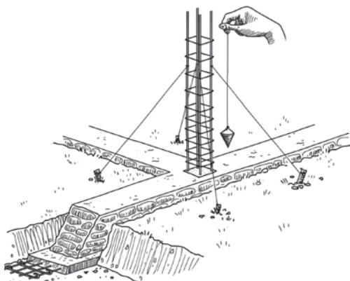
Leave a space around the reinforcement for the concrete.
