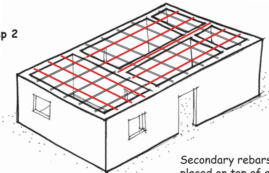
Secondary rebars are placed on top of and perpendicular to the primary rebars.
