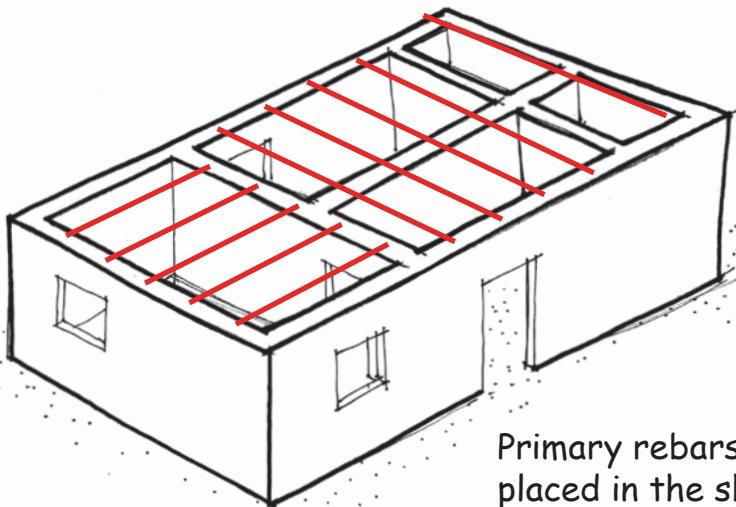
Primary rebars are placed in the shorter direction (span).
