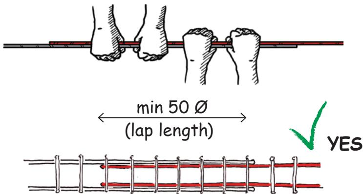
Tie wires only hold the rebars in place. They don't add strength to the connections!
