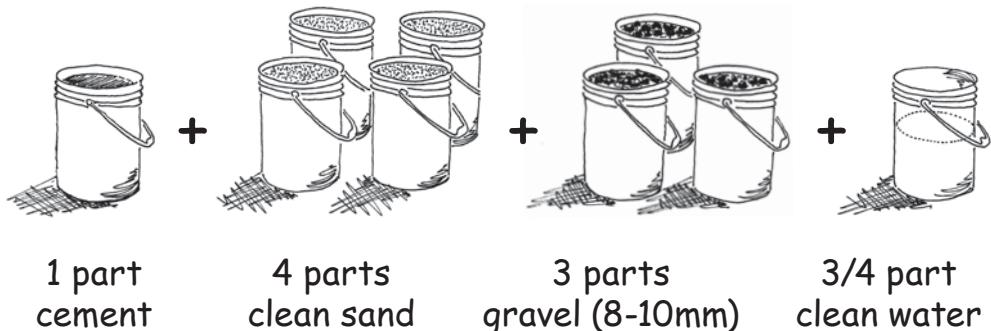
Sand should be crushed, washed and dried.
