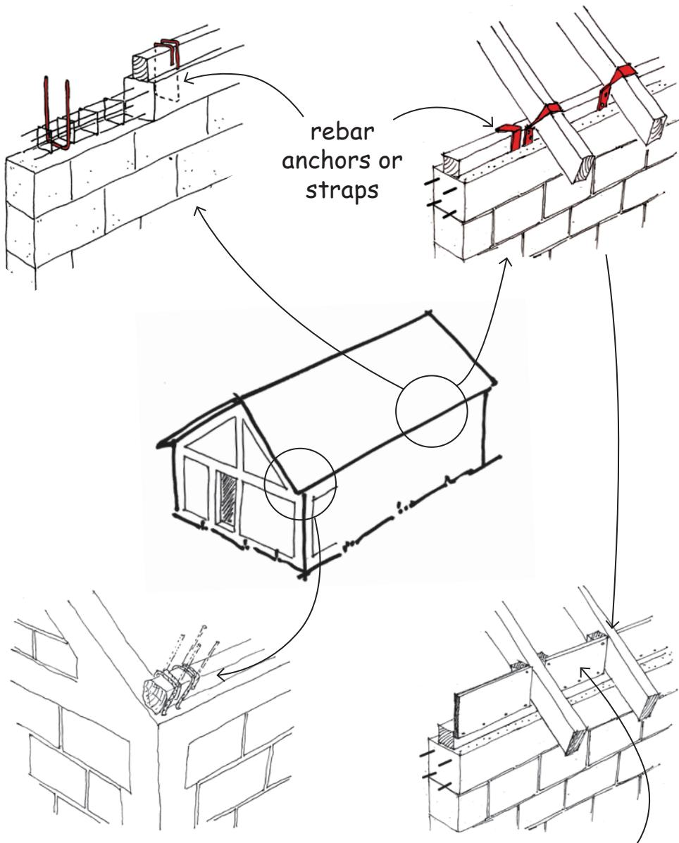
Solidly fasten the anchors or straps to the wood framing.
