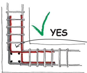
Put an additional rebar around the outer corner.
