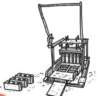
To compact the concrete, hit the mold with a shovel and a hammer.
