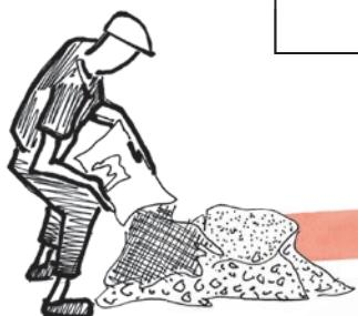
1. Make a pile with the gravel, the sand and the cement but without water.
