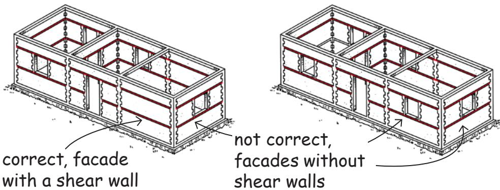
In these cases shear walls are created by increasing the reinforcements on the side of some specific openings.
