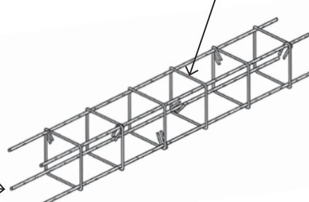
Rebar dimensions for vertical and horizontal ties
