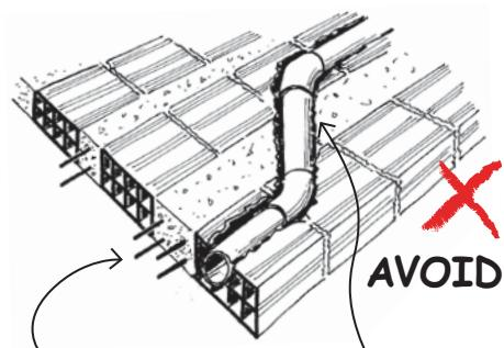
Pass pipes through the hollow blocks and through concrete only in one spot. Reinforce joist with additional rebars.
