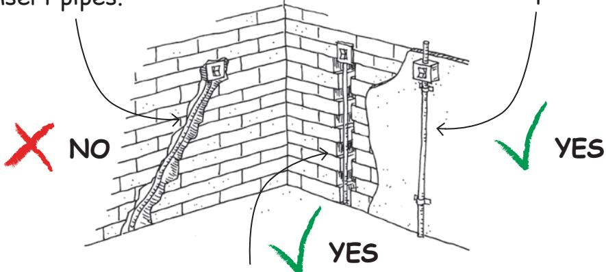
Leave a space in the wall for electrical pipes.
