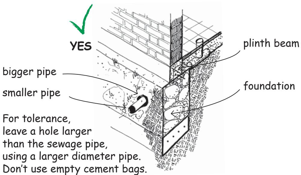
The pipe must go through the foundation, under the plinth beam.
