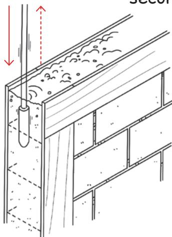
Advance at regular intervals following the action radius of the needle.
