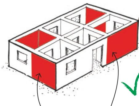
Each facade must have at least one tied wall without openings. These are shear walls.
