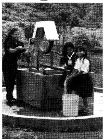
The rope pump has proven to be a sustainable option for rural water supply, used at family and community level and delivering water to already more than 10 % of the rural population in Nicaragua with over 12.000 units installed. It is the national standard for the rural water and sanitation sector.
