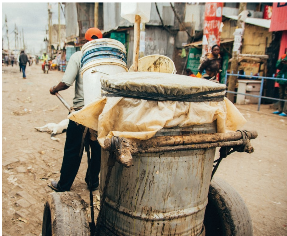
Photo 1 Ambulances used by manual pit emptiers to transport latrine contents. Placing the barrels on modified handcarts warps the barrel shape. Lids no longer fit, and emptiers use tarps to contain the contents of the barrel
