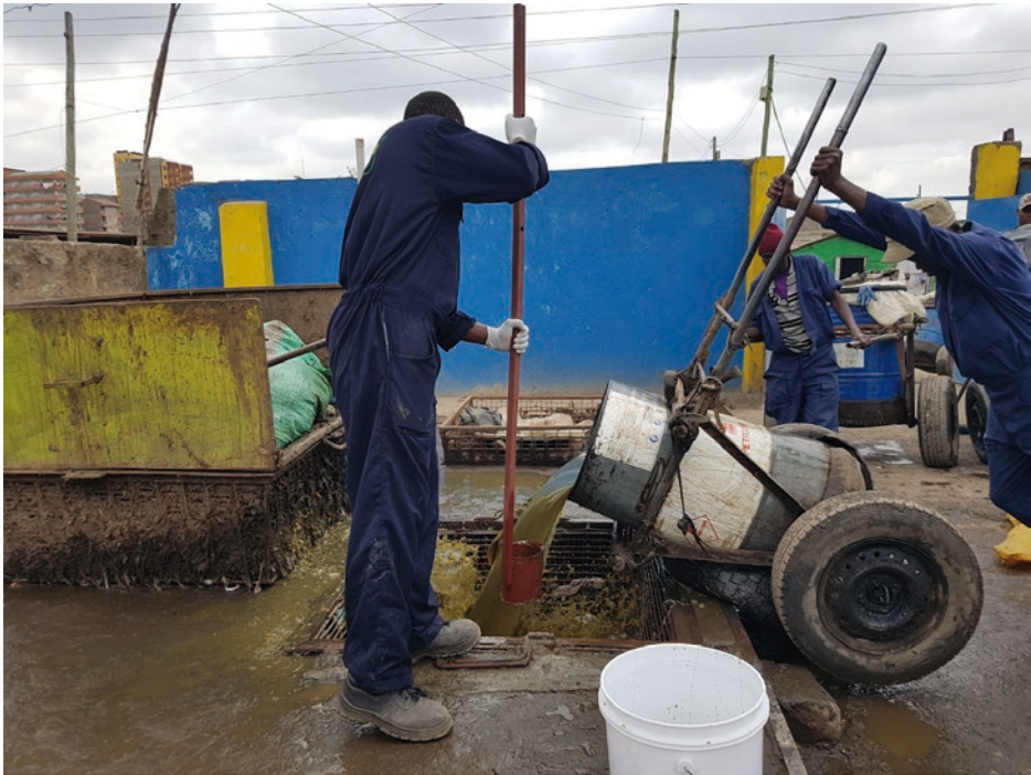
Photo 2 Pit emptiers tipping their ambulances into the holding tank through the double-mesh screen while the transfer station operator collects faecal sludge for a laboratory study. Transfer station operators use water to flush any spills back into the holding tank
