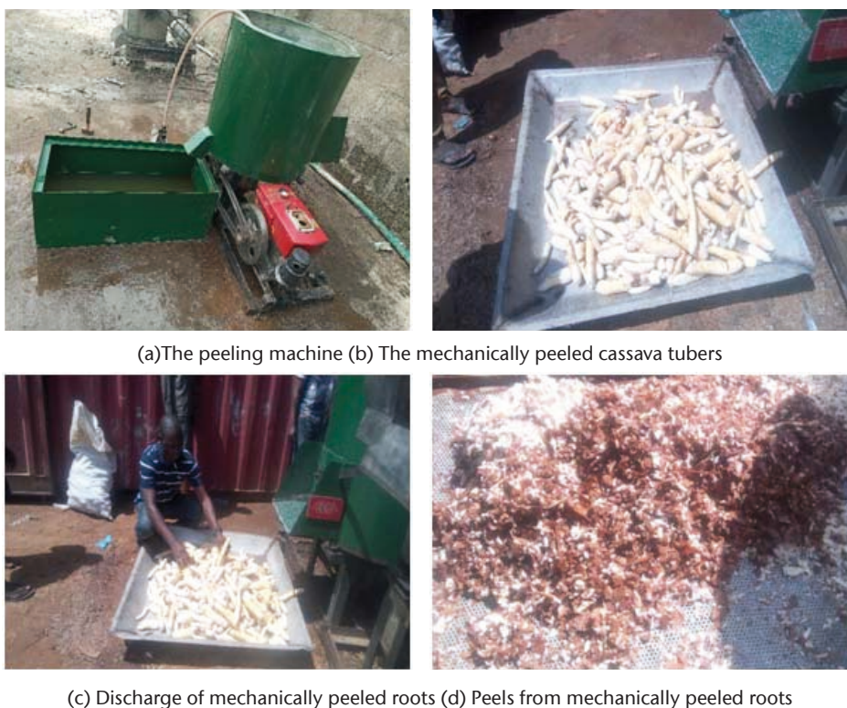
Photo 1 Peeling machine, peeled roots, and the peels
