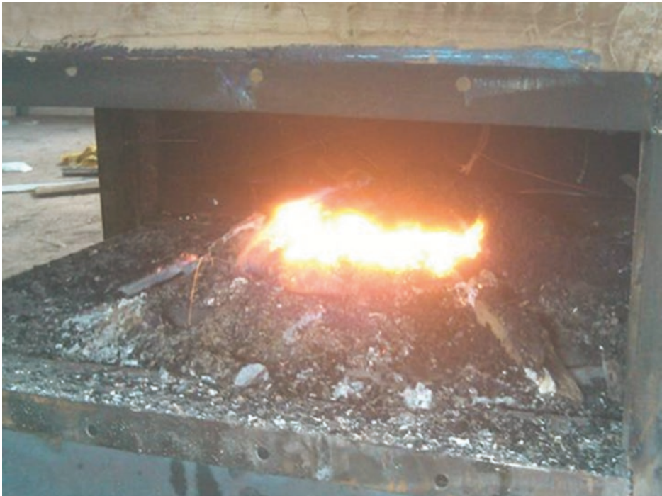
Figure 2 Classic combustion pattern showing drying phase (unburnt) in centre, and then outwards to volatiles and char combustion, and ash lower down (wood is residue from start-up)
