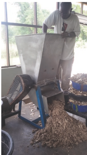
Figure 2 Modified grater for cassava peels
