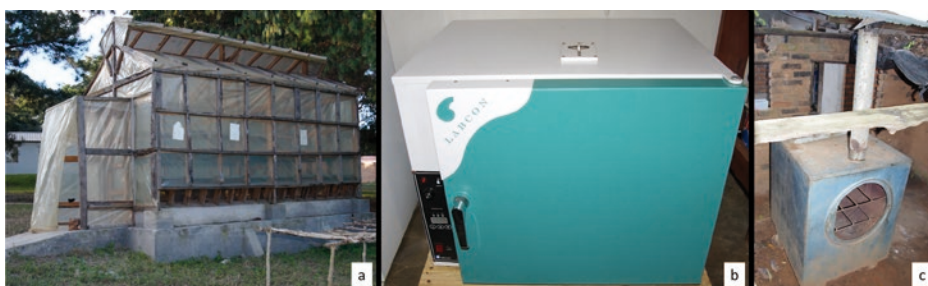
Figure 1 Drying methods used in this study: (a) solar dehydrator; (b) electric oven; (c) wood-fired drum oven
