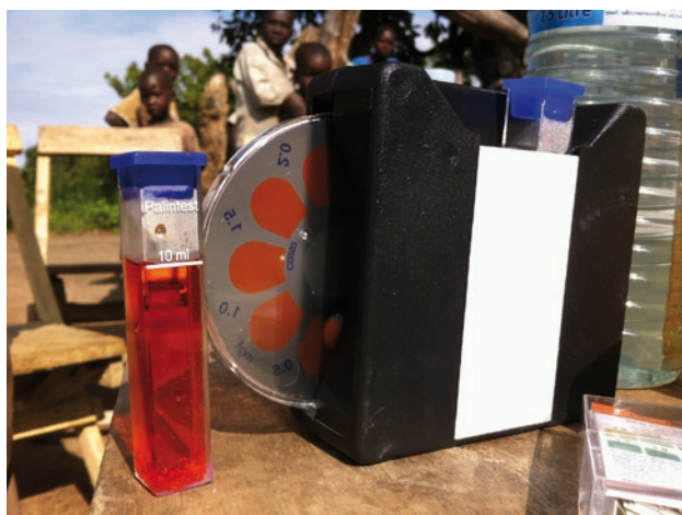
Figure 2 Palintest comparator test kit
