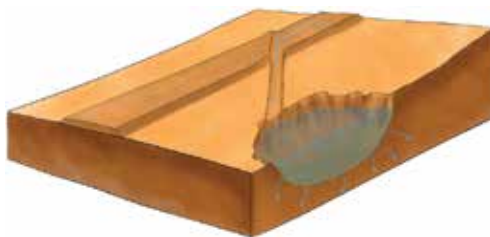
Figure 3 Rolling dip evacuating runoff generated by road to nearby pond
