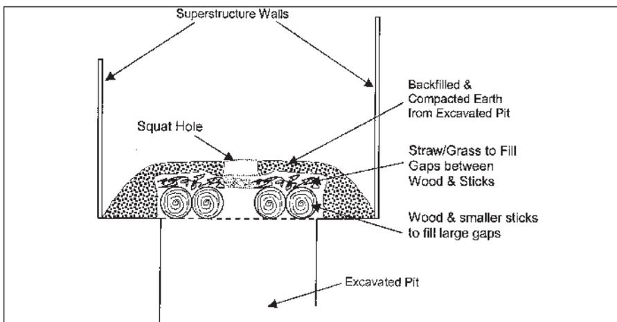
Figure 1. The Oxfam pilot design for a latrine
